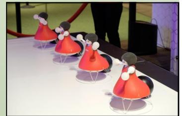
The robots sit on top of balls and use advanced sensing, communication, and group control technologies to stay balanced as they quickly move and dance around. The robot cheerleaders were developed by a team of 21 engineers and scientists who worked for over two years to create the robots, which had to be synchronized through special technologies so they can dance in unison.
